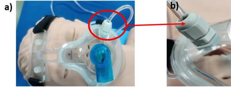
a) Prototype NIV mask placed on mannequin b) Gland nut mechanism for feeding port
